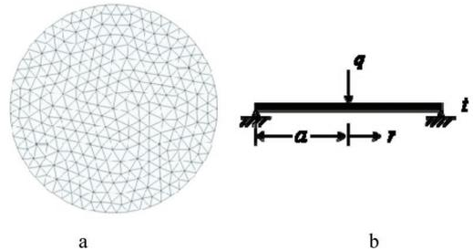
Figure 4. Geometry of circular plate: a. elevation of the mesh; b. side view.
