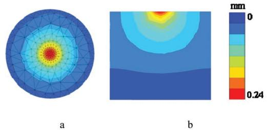
Figure 13. Contour plots of settlement: a. top view; b. cross section through problem ( $E_2 = 20000 \text{ kN/m}^2$ ).
