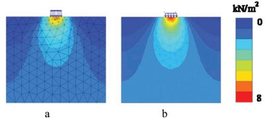
Figure 8. Contour plots of vertical stress in the soil below loaded plate: a. results using implemented plate element; b. results using Plaxis.
