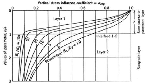
Figure 11. Vertical stresses in a two layer system (Burmister, 1958).
