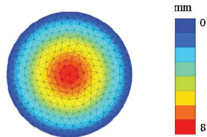
Figure 6. Contour plot of deflection of the circular plate.
