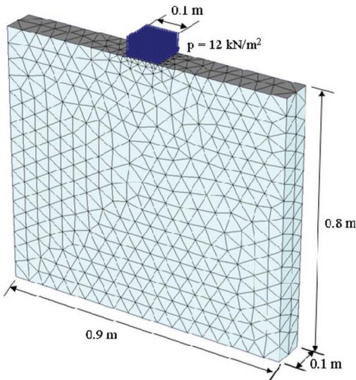
Figure 7. Geometry of centrally loaded plate resting on elastic foundation.
