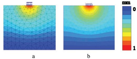
Figure 9. Contour plots of vertical displacement in the soil below loaded plate: a. results using implemented plate element; b. results using Plaxis.
