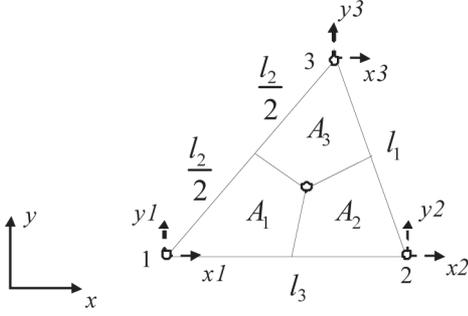
Figure 2. Mass lumping for 3-node triangular plate element.
