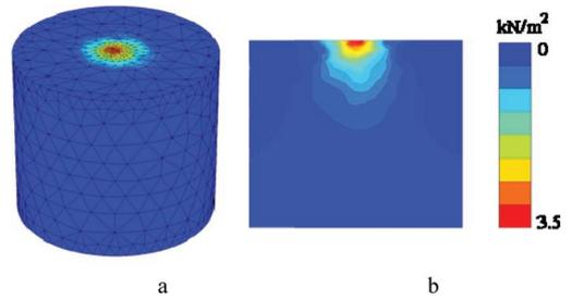
Figure 12. Contour plots of vertical stress: a. 3D view; b. cross section through problem ( $E_2 = 20000 \text{ kN/m}^2$ ).
