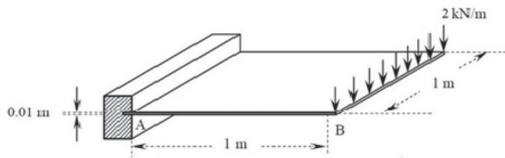
Figure 3. Cantilever plate subjected to a uniform end load.
