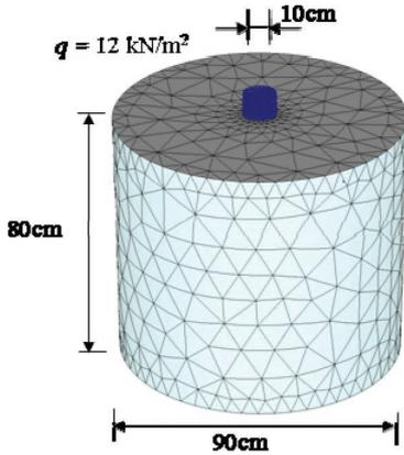
Figure 10. Geometry of loaded plate resting on half space.
