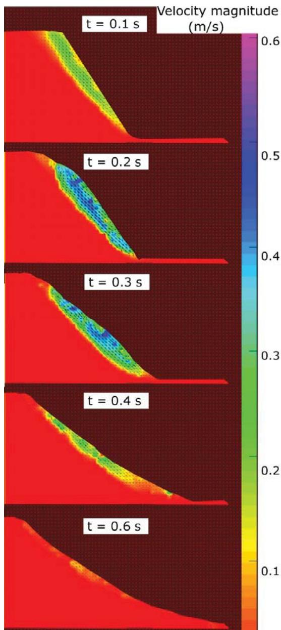
Figure 4. Velocity maps derived from the digital imaging of the failure induced in a  $60^\circ$  sand slope using a PIV technique. The color indicates the magnitude of the displacement velocity vector of each point.
