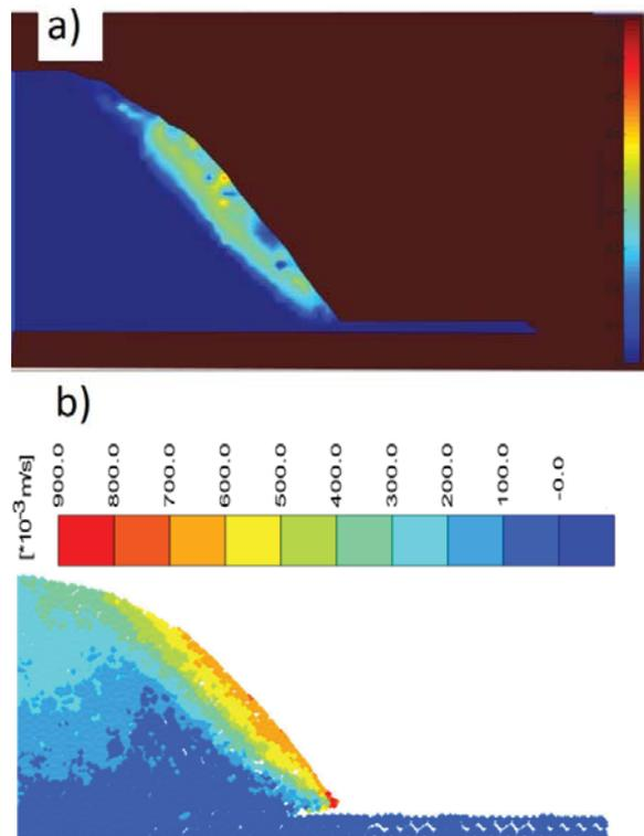
Figure 7. Comparison between experimental (a) and numerical (b) results of the velocity magnitude distribution at  $t = 0.22s$ .
