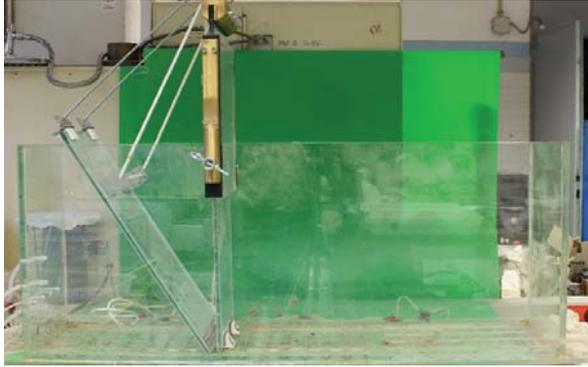
Figure 1. Tank showing the guillotine and water injection system to perform the scaled landslides.
