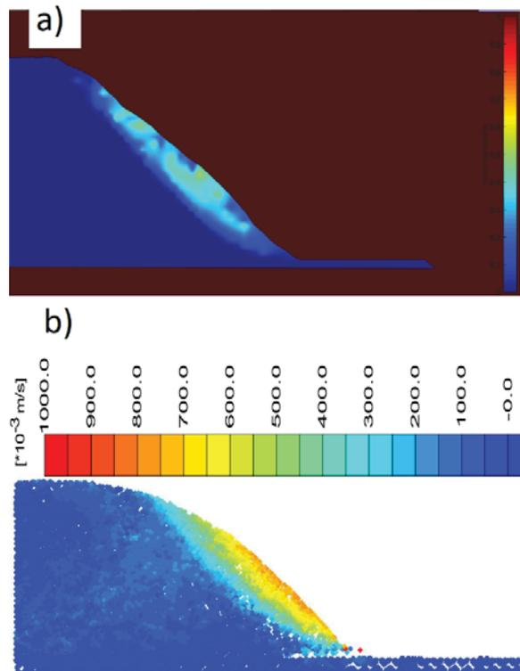
Figure 8. Comparison between experimental (a) and numerical (b) results of the velocity magnitude distribution at  $t = 0.28s$ .
