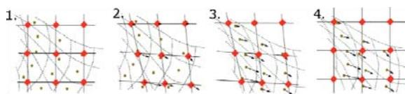
Figure 3. Scheme of the computational sequence in MPM. Material points (brown), grid nodes (red).
