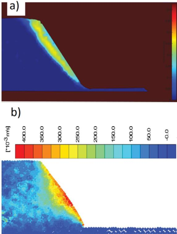
Figure 5. Comparison between experimental (a) and numerical (b) results of the velocity magnitude distribution at  $t = 0.1s$ .
