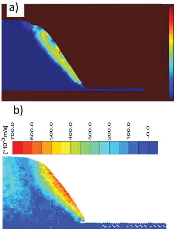
Figure 6. Comparison between experimental (a) and numerical (b) results of the velocity magnitude distribution at  $t = 0.16s$ .
