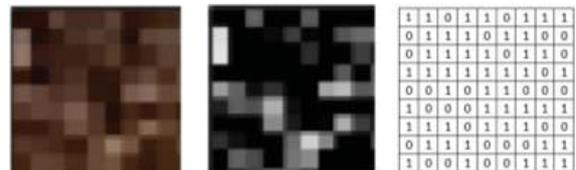
Figure 2. Ideal example of a codification in patterns in the PIV technique. Left: digital picture; center: simplified gray scaled picture; right: binary code.
